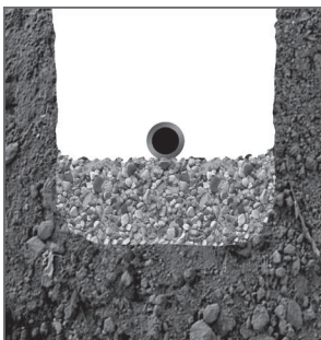
Trench in bad soil
